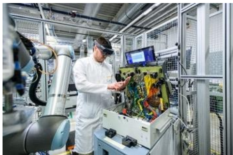
Figure 20: Assisted maintenance of production equipment using augmented reality and 5G. Source: AYES Archive, 2023.
